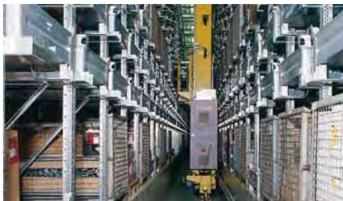
Automated pallet racking with single position storage
