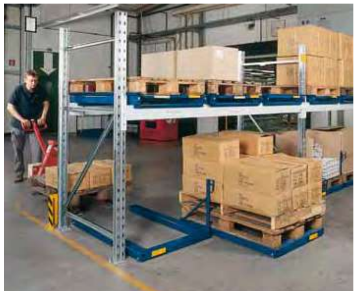
Floor mounted and beam mounted extraction units
